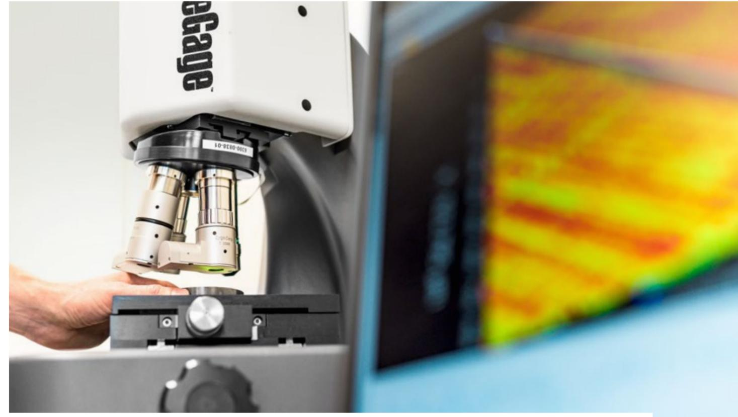
*Efficient control of the machine and contactless optical measurement ensure that the surface quality of the processed workpieces is high.*
